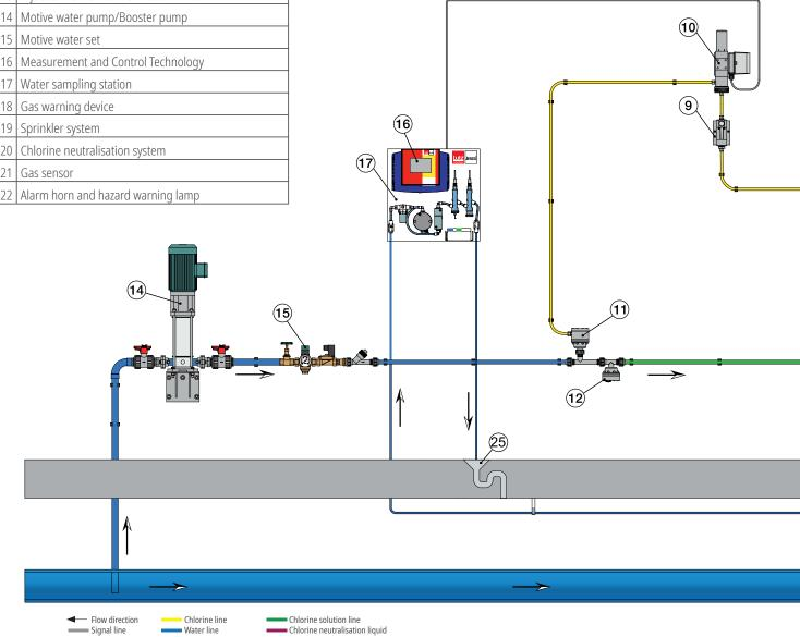
Example of a chlorinator with gas take-off up to 10 kg  $Cl_2/h$  under a vacuum with neutralisation system (installation example: removal 1.3 kg  $Cl_2/h$ , max. 2.6 kg  $Cl_2/h$ )
