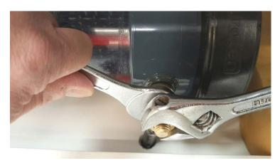
Place a 19mm spanner on the thin locking nut and an adjustable spanner on the front cable securing nut. Take care to hold the locking nut steady whilst turning the front securing nut anti-clockwise to loosen it. Repeat this procedure on the remaining terminal and remove the brass nuts and washers for safe keeping. Ease away the cable lugs from the threaded terminal bar; the cable glands
