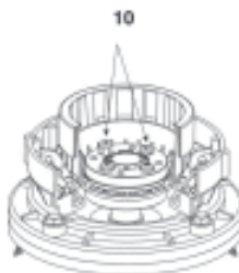
Fig. 8.1.2 G - Disassembly of the drive magnetic assembly
