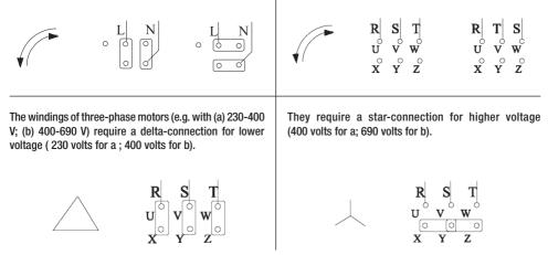
Star/Delta starting is used when the motor power is above 7.5 kW (10 HP) only in case of frequent starts and short running times, but always when the motor power is above 15kW (20 HP). All this is also to safeguard the structure of the pump.
