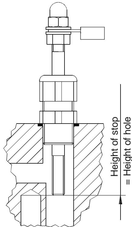
If the switching function is still not correct after adjusting the upper stop, the Reed contact can be shifted in the screw terminal in order to obtain a precise adjustment.
