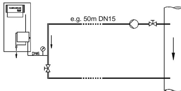
The pump conveys the water over this long distance in a loop line past the water sampling station and only part of the water flow is used for the actual measurement. Under no circumstances should the butterfly valve be fully closed, otherwise long delays can make control more difficult. Moreover, the water would heat up strongly in the pump, thus also leading to measurement errors. A pressure gauge in the loop line is useful for adjusting the butterfly valve.
