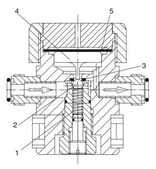
The liquid coming from left first faces a shut valve (ball/seat 2+3) which is closed by the spring (1) and sealed additionally by the liquid pressure. Thus liquid can only flow if the ball (2) is pushed down by the plunger (4). This happens only after a vacuum has been produced at the right connection due to the suction stroke of the pump, causing the diaphrgam (5) to move downwards and press with the plunger (4) onto the ball (2).
