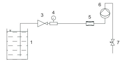
d) Protection of the metering pump against pressure peaks due to acceleration in the case of long suction lines.
