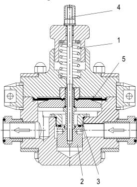
The liquid coming from right first faces a shut valve (valve head/valve seat 2+3) which is closed by the spring (1) and sealed additionally by the liquid pressure. Thus liquid can only flow if the valve head (2) is pushed down by the valve pin (4). This happens only after a vacuum has been produced at the left connection due to the suction stroke of the pump, causing the diaphragm (5) to move downwards and thus lift the valve head (2) off the valve seat (3).
