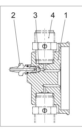
The quantity of leakage is dependent on operating pressure: if this is subject to fluctuation the constancy of the leakage and thus of the dosing itself can be improved by installing a back-pressure valve in the pressure line. This valve should be set at approximately 0,5 bar above the highest foreseeable operating pressure.
