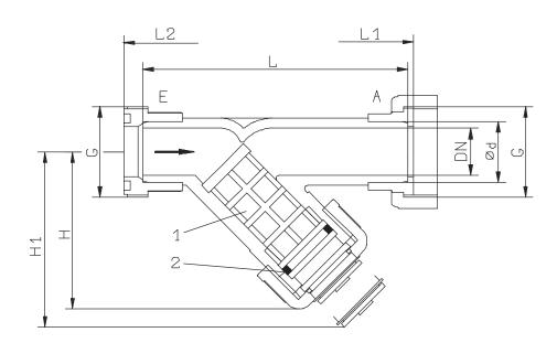
The dirt trap shown here is made of transparent PVC and has cemented connecting pieces on both sides. Upon request, it can be supplied with threaded parts (see "E") or with adjusting parts (see "A").
