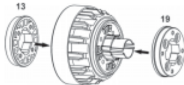
Fig. 8.3.2 B - Assembly of the collars
