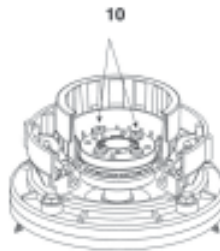
Fig. 8.1.2 G - Disassembly of the drive magnetic assembly
