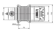
Fig. 6: Dimensioned drawing of MEMDOS SMART LK / LP 2, 5, 10 with dosing head made of PVC, PP or PVDF (all dimensions in mm)
