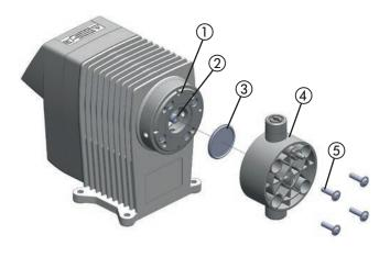
Fig. 53: Exploded view of the diaphragm and dosing head
