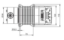
Fig. 8: Dimensioned drawing of MEMDOS SMART LK / LP 15, 20, 30 with dosing head made of PVC, PP, PVDF or stainless steel (1.4571) (all dimensions in mm)
