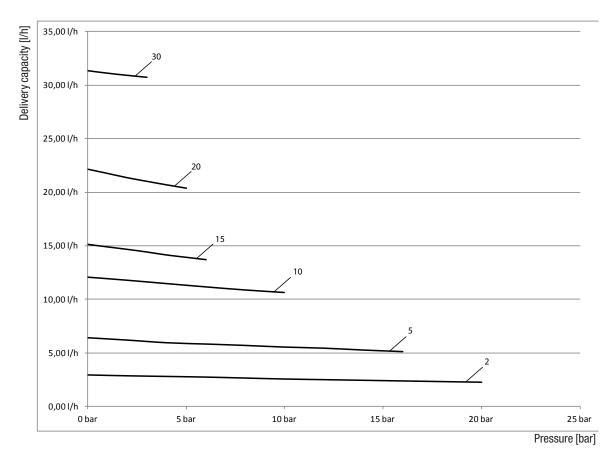
Fig. 57: Delivery characteristic curves MEMDOS SMART LK / LP 2 - 30
