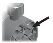
Fig. 17: Dosing head venting facility with hose connection
