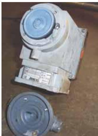
Destroyed solenoid-driven diaphragm dosing pump MAGDOS E.
