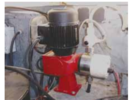
Now applied: special MEMDOS E with heated dosing head.
